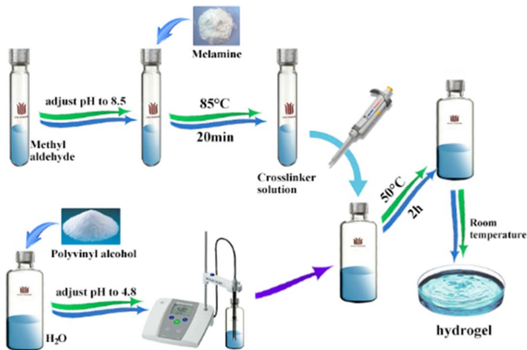
Figure 2. Schematic diagram of PVA hydrogels preparation. [Color figure can be viewed in the online issue, which is available at wileyonlinelibrary.com.]
