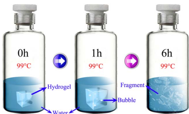
Figure 4. The PVA hydrogel changed from block to fragment at 99°C. [Color figure can be viewed in the online issue, which is available at wileyonlinelibrary.com .]
